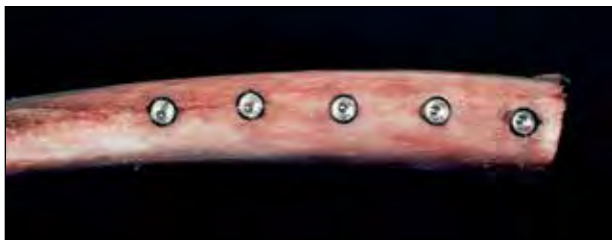
Fig 1 Five implants were positioned in each cow rib, with 20 mm between each implant.
