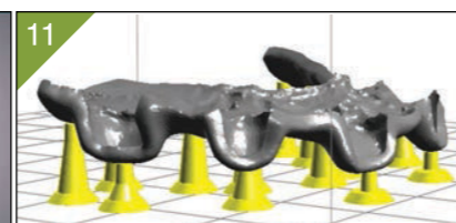
Figure 11. Jig positioned on the Zenith software with virtual support for printing.
